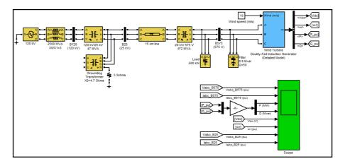
Fig. 3 The DFIG simulink model
