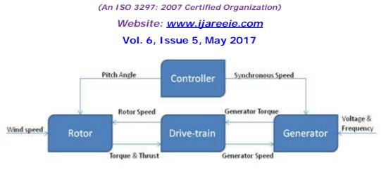
Fig. 1 The Block diagram of Wind Energy Conversion System
