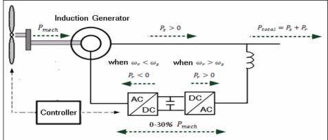
Fig. 2 The Block diagram of DFIG System
